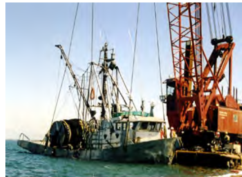
Photo 5. The 14.7 m Cap Rouge II alongside the salvage barge after being righted from the capsized position
