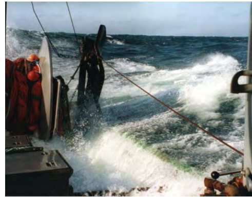
Photo 4. A wave breaks over the bulwarks and fills the deck, showing the importance of watertight deck integrity
