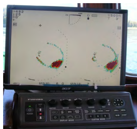
Photo 12. A dual scanning sonar showing the seine and the catch of sardines
