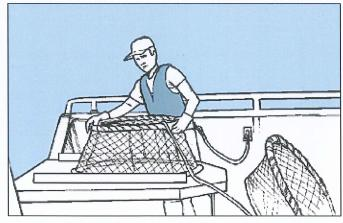
Crew working on the stern, where they are snapping black cod traps to the ground line, must wear a safety belt or a harness and be secured to a lifeline.
